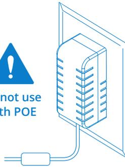
Plug in power adapter to wall outlet and connect Ethernet cable if applicable.
