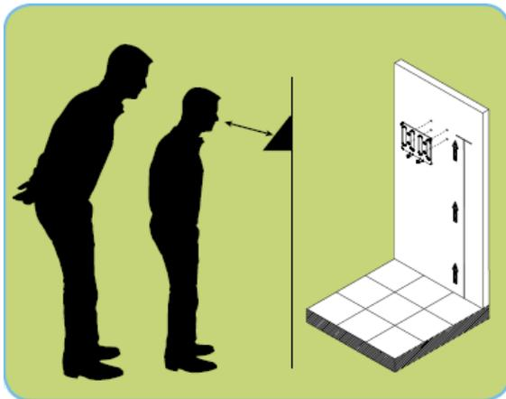
Install the mounting-plate to the wall using the supplied screws. For sheetrock walls, drill a 3/16" diameter hole through each of the four screw locations; each approx 1-1/2" deep. Install the plastic "anchors" included in the mounting screw packet.
