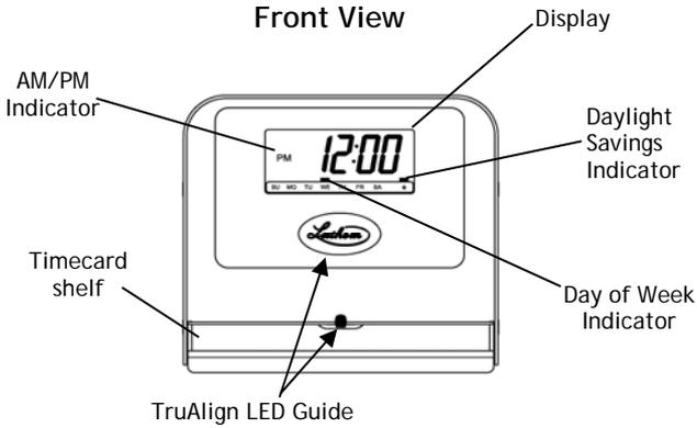
The employee places the long edge of the timecard on the timecard shelf of the 800P and aligns the timecard to the cell to be printed. When the timecard is aligned correctly an automatic imprint with the day and time will be recorded on the timecard.
