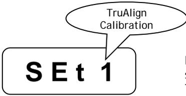
Press the **+** or **-** button until the display shows '1'. Selecting '1' activates the TruAlign calibration mode. Press the **SET** button.
