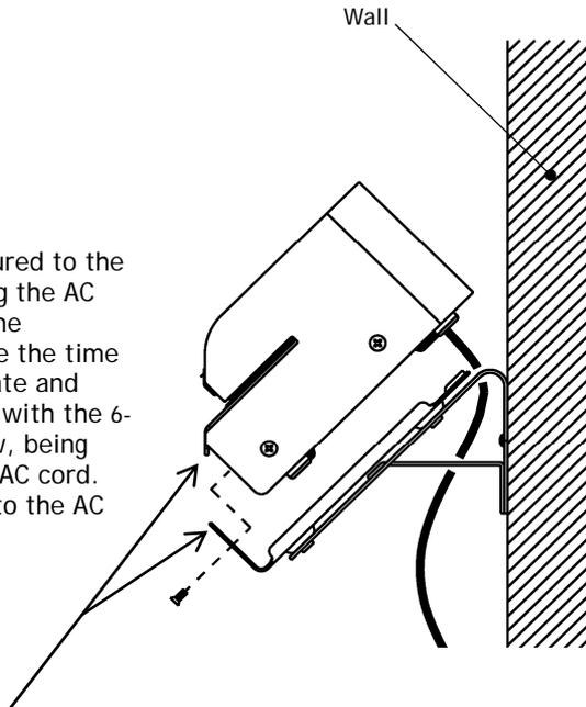
**Note:** Make sure the bottom of the timecard shelf is over the edge of the back-plate before securing the screw.
