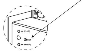
**Note**: Normally you would use the default settings and by pass the Daylight Savings settings by pressing the **SET** button.
