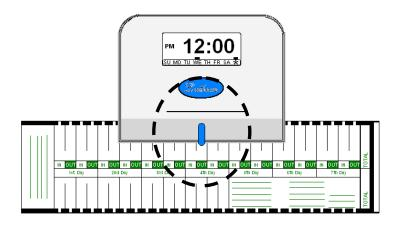
Next, four dashes (- - - -) show on the display and the indicator turns green indicating the printing is complete and the timecard can be removed.
