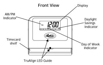
The employee places the long edge of the timecard on the timecard shelf of the 800P and aligns the timecard to the cell to be printed. When the timecard is aligned correctly an automatic imprint with the day and time will be recorded on the timecard.
