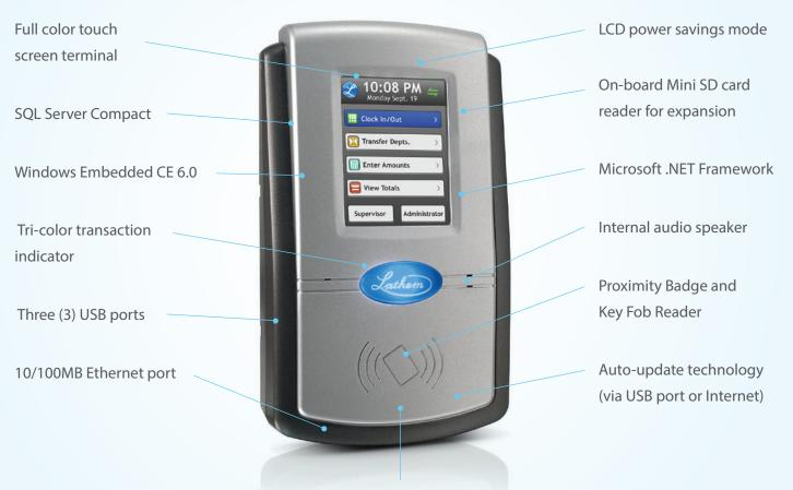
Internal dry contact provides access control and bell ringer capabilities
