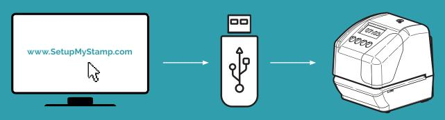
All print formats and custom text messages can be configured online and programmed to the unit using a standard USB flash drive eliminating complex button setup.
